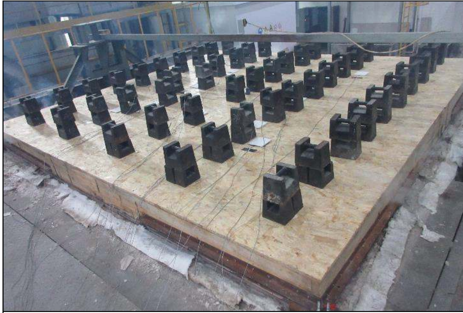
The unexposed face after test duration of 120 minutes
