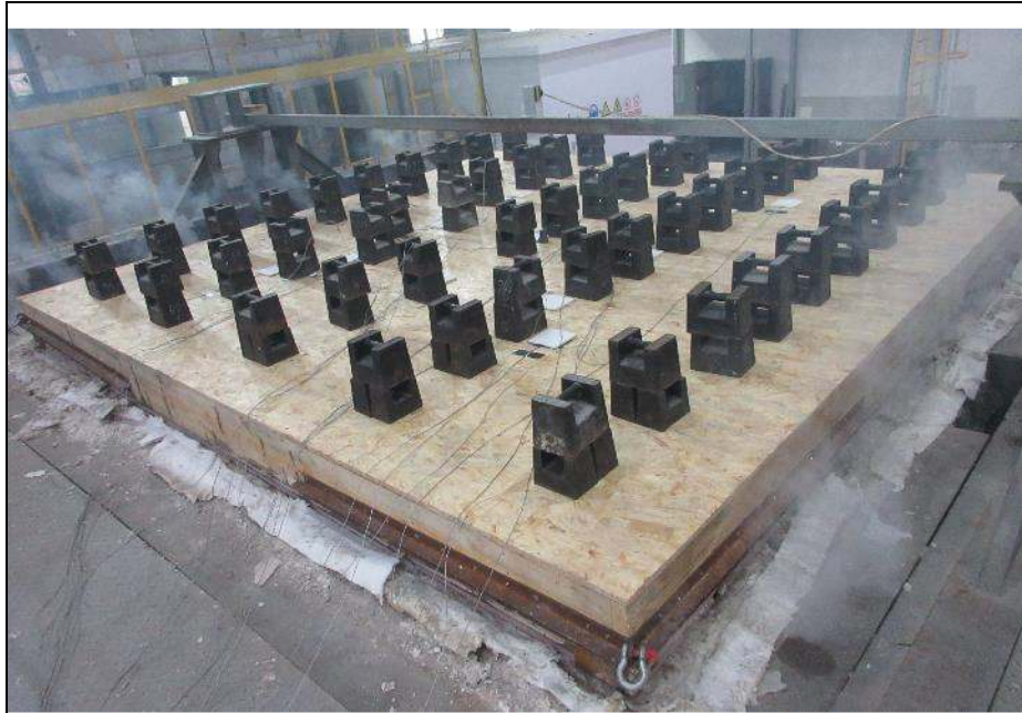
The unexposed face after test duration of 40 minutes
