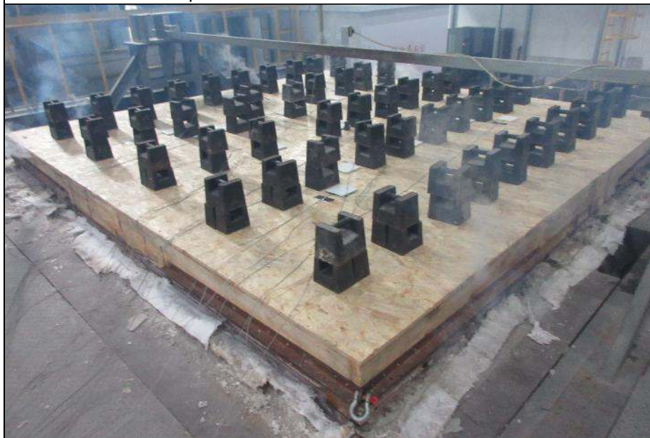
The unexposed face after test duration of 92 minutes
